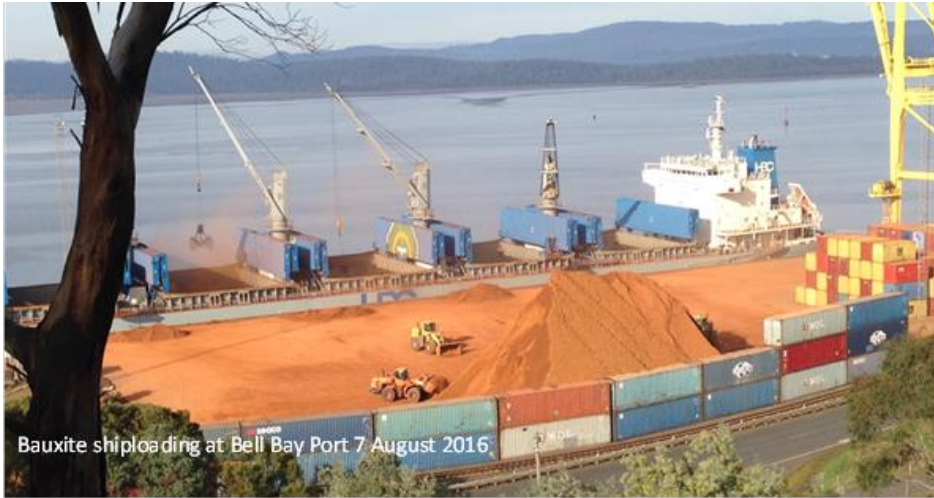
Figure 8 Loading 35,500 tonnes of bauxite at Bell Bay port Bell Bay port can handle ships up to 65,000 tonnes.
