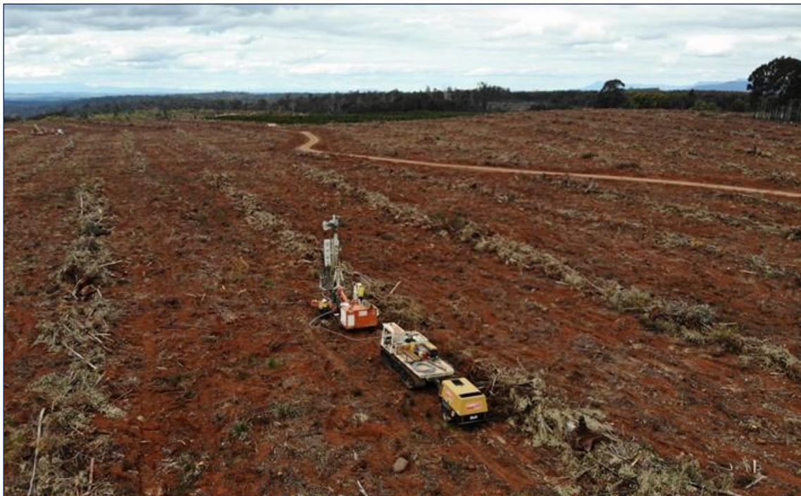
Figure 4: Drilling the eastern flank of the Deep Leads REE discovery. The equipment is designed to fit between plantation hardwood trees which in this case, have just been harvested.
