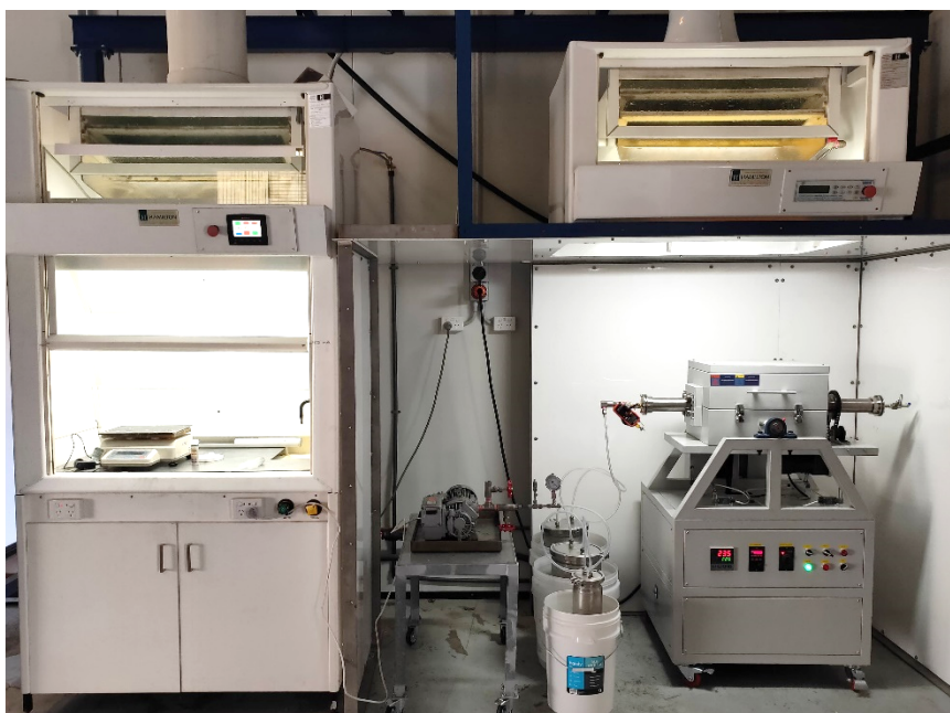
Figure 2: Alcore specialised laboratory reactor to react oleum with bath to recover fluorine
