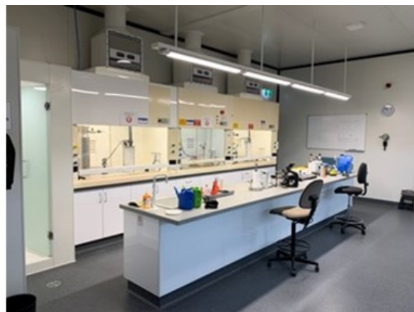
Figure 10 Alcore test lab, fume cabinets with hi-tech fume scrubbers, showers, microscopes & Draegar air monitor (far wall)
