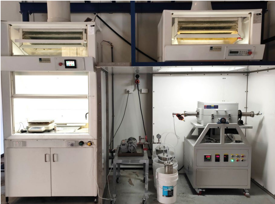
Rotary kiln for recovery of fluorine from aluminium smelter bath
