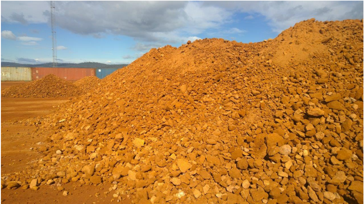
Figure 3: ABx blends the product at the mine site and loads onto the port stockpile to maximise mixing during reclamation and ship loading. During ship loading at Bell Bay and again at unloading, this stockpile will be mixed further, thus providing a consistent product. Note that the containers in the background are used by the Stevedoring company as a dust barrier to avoid cross-contamination with other cargoes and are not involved in the bulk shipment of ABx bauxite.
