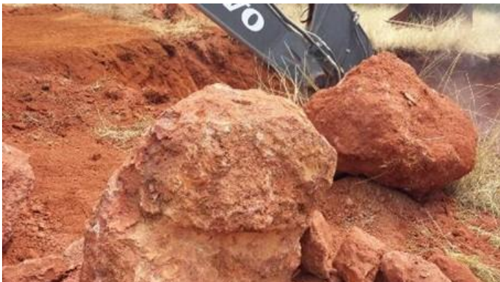
Figure 13 Best ore comes as blocks which need crushing Grades exceed +50% \text{Al}_2\text{O}_3 and less than 2% \text{SiO}_2
