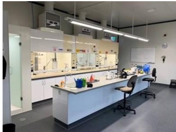
Figure 5 ALCORE test lab, fume cabinets with hi-tech fume scrubbers, showers, microscopes & Draeger air monitor (far wall)
