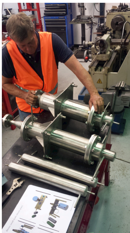
Figure 2: Pilot scale reactors for production of precursor chemicals
