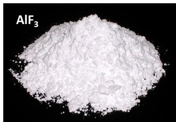
Figures 1, 2 & 3: AlF 3 is added daily into aluminium smelter potlines to maintain efficiency. There is no substitute. Australia is the only major aluminium producer without an AlF 3 plant. Alcore will secure supply and help recycling.
