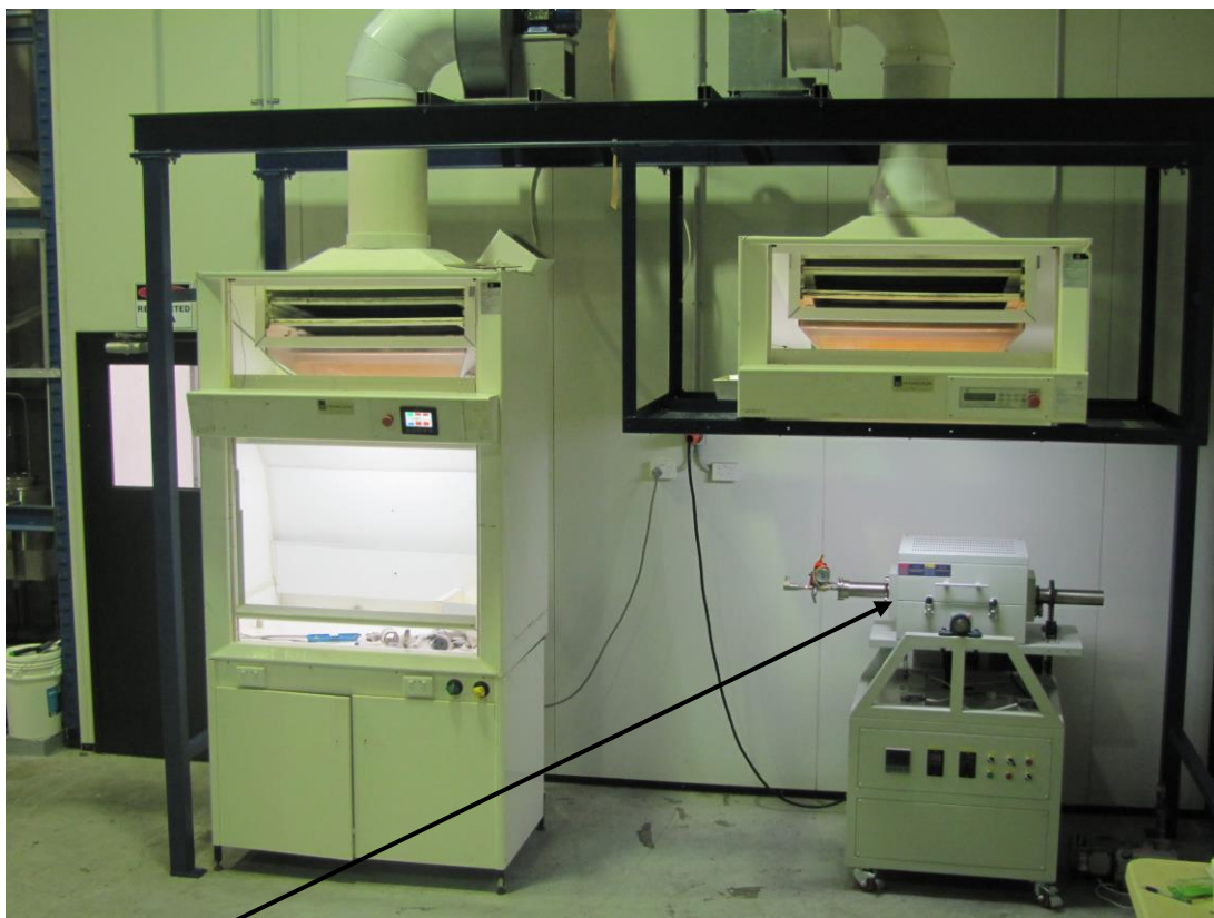
Figure 5: Customised reactor for further testing of the recovery of fluorine from aluminium smelter bath
