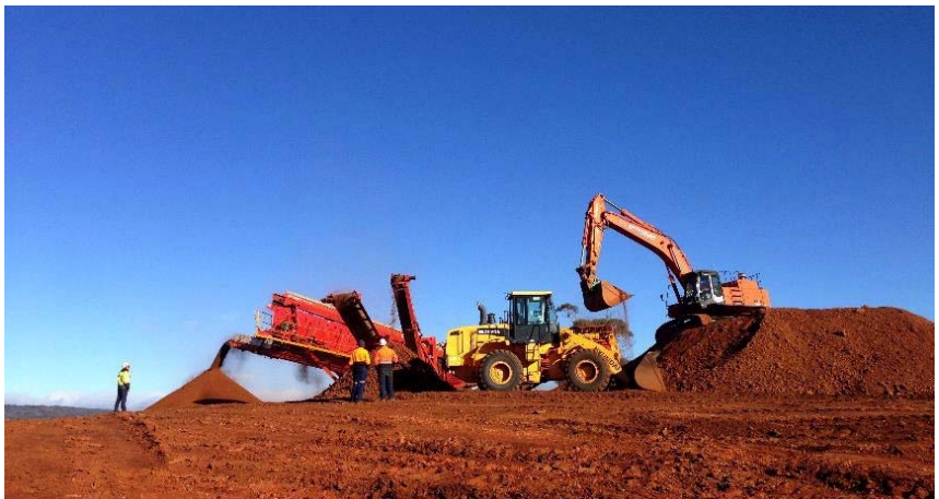
Figures 3 & 4 (below): Bench mining pit MB3. Feeding dried ore to screen at MB5
