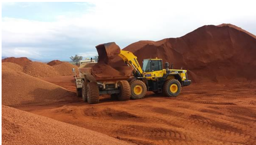
Figure 4 Blending 33,000 tonnes of cement-grade bauxite at Bald Hill Mine Site
